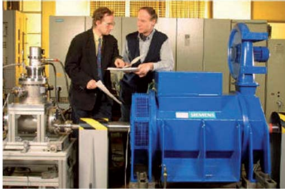
Fig. 8.16. Siemens 400 kW HTS synchronous machine in the test bed. Photo courtesy of Siemens [135, 136].
