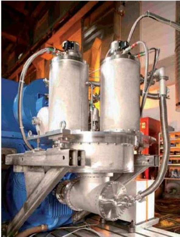
Fig. 8.18. Cryogenic cooling system of the 4 MVA Siemens HTS generator. The third refrigerator is hidden behind the right one. Photo courtesy of Siemens .
