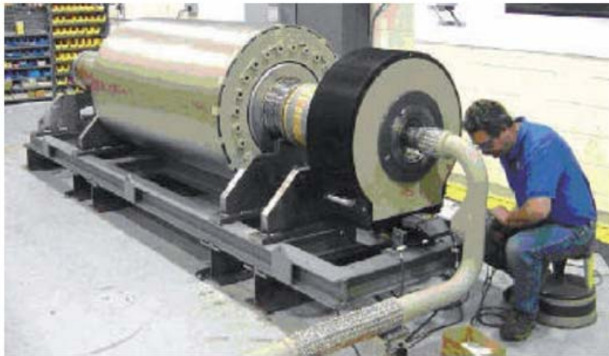
Fig. 8.6. BSCCO HTS rotor assembly with exciter of the 5 MW synchronous motor manufactured by American Superconductors [9].
